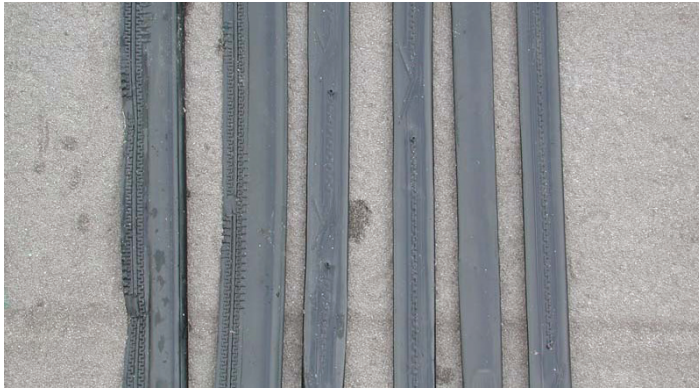
Figure 3. Drip tapes can be distinguished and recognized by their features. Note the emitter (on the four tapes on the right) and the turbulent flow channels (on the two tapes on the left). Credits: Eric Simonne.
