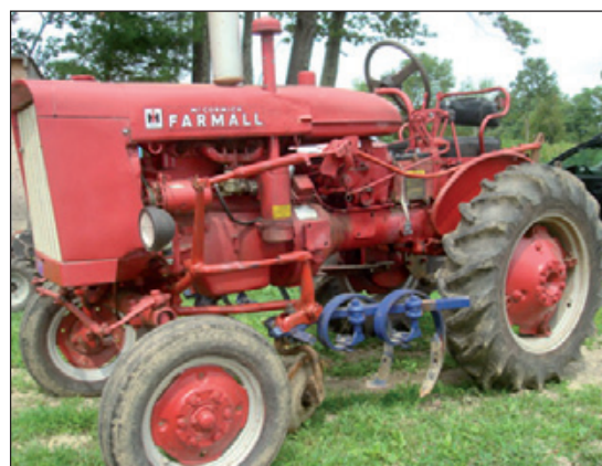
The author's Farmall 140 with belly-mounted implements. Photo: Andy Pressman, NCAT
