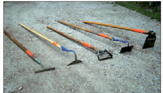
From left to right, a collinear hoe, a swan-neck hoe, a stirrup hoe, a “regular” hoe, and an eye-hoe. Photo: Andy Pressman, NCAT
