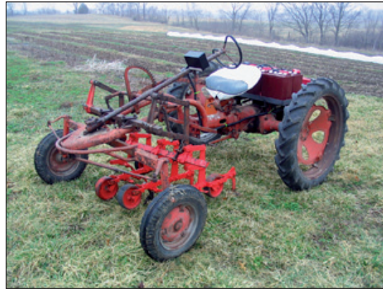
An Allis Chalmers G converted to electric at Fair Share Farm, Kearney, Missouri. Photo: Rex Dufour, NCAT
