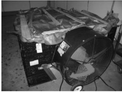
Figure 1. An inexpensive, home -made, forced-air cooling set up.
