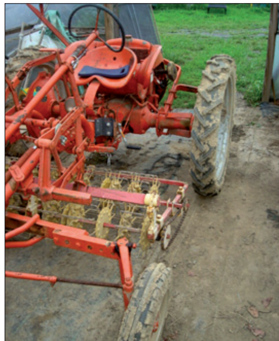
A basket weeder belly mounted to an Allis Chalmers G at Pennypack Farm and Education Center in Horsham, Pennsylvania. Photo: Andy Pressman, NCAT
