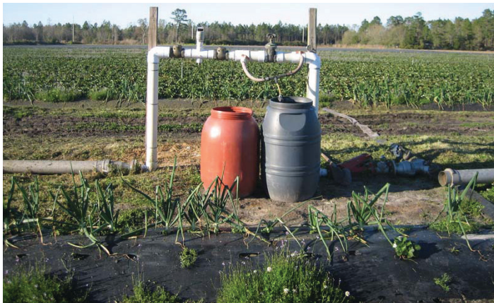
Figure 4. Back-flow prevention made of two ball valves and a vacuum breaker are placed upstream of the Venturi injector. Credits: Eric Simonne.
