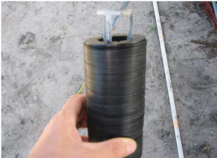
Figure 6. Disk filters are made of stacked disks with small openings. They are usually color coded to indicate the filtration mesh. Credits: Eric Simonne.
