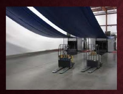
This method also requires a cold chamber, but also uses fans, tarps, and a system of air ducts to <u>force cold air</u> <u>directly through produce containers</u>.
